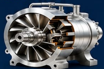
Centrifugal Compressor - Cutaway View
